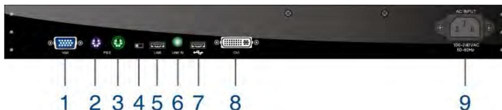
**Figure 3-2. The Rear View of Single Port LCD Console**
